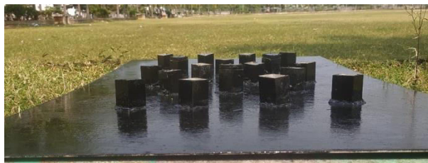
Fig. 2. Fabricated Rhombus Wax Storage Unit (RWSU) bonded to the absorber plate.
