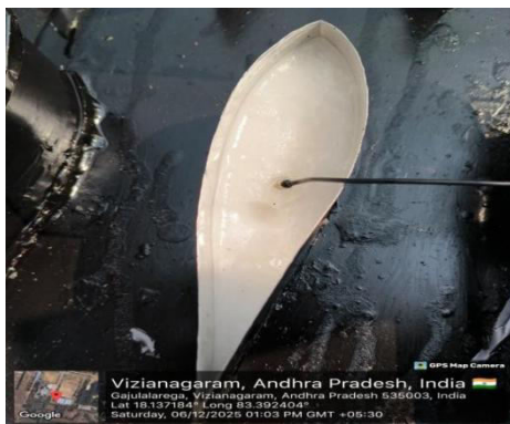
Fig. 3. Wax-filled Aerofoil Wax Storage Unit (AWSU).
