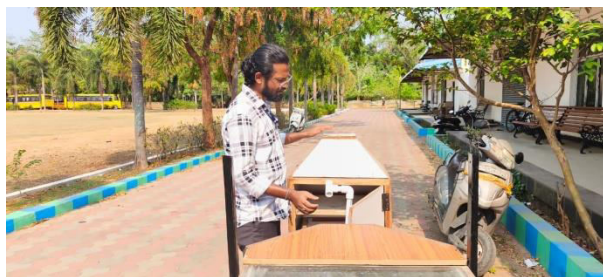
Fig. 4. Fabricated experimental solar dryer test rig.
